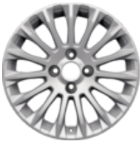
Alloy Wheel 16" 15-spoke design, silver Single alloy wheel, 6.5j x 16", offset 40, fit with 195/55 R16 tyre
