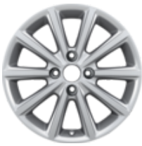
Alloy Wheel 16" 10-spoke design, silver Single alloy wheel, 6.5j x 16", offset 40, fit with 195/55 R16 tyre
