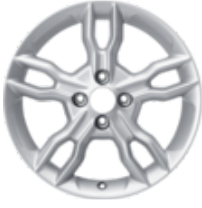
Alloy Wheel 16" 5 x 2-spoke design, sparkle silver Single alloy wheel, 6.5j x 16", offset 40, fit with 195/55 R16 tyre
