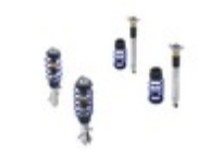
Coilover Suspension Kit stainless steel with powder coated springs in Ford Performance blue
