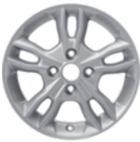
Alloy Wheel 15" Alloy Wheel 15" 5 x 2-spoke design, sparkle silver Single alloy wheel, 6j x 15", offset 47.5, fit with 195/55 R15 tyre – Except ST
