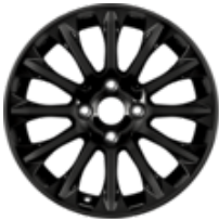
Alloy Wheel 16" 12-spoke design, Panther Black Single alloy wheel, 6.5j x 16", offset 47.5, fit with 195/45R16 or 195/50R16 tyre
