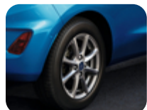
Alloy Wheel 15" 8-spoke design, Sparkle Silver Single alloy wheel, 6j x 15", offset 45, 195/60 R15 tyre (not included)
