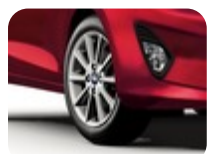
Alloy Wheel 16" 10-spoke design, Sparkle Silver Single alloy wheel, 6.5j x 16", offset 47.5, fit with 195/55 R16 tyre
