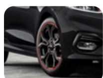
Alloy Wheel 17" 5 x 2-spoke Y design, Black with red accent ring Single alloy wheel, 7j x 17", offset 47.5, fit with 205/45 R17 tyre
