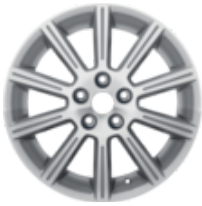
Alloy Wheel 17" 10-spoke design, silver Single alloy wheel, 7j x 17", offset 55, fit with 225/50 R17 tyre – Only in combination with steering rack limiter, from 2006 onwards
