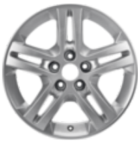
Alloy Wheel 16" 5 x 2-spoke design, silver Single alloy wheel, 6.5j x 16", offset 50, fit with 215/60 R16 tyre – from 2006 onwards
