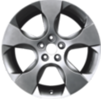
Alloy Wheel 18" 5-spoke design, Mystique Silver Single alloy wheel, 8j x 18", offset 55, fit with 235/45 R18 tyre – Only in combination with steering rack limiter, from 2006 onwards
