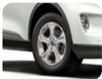
Alloy Wheel 17" 5-spoke design, Shadow Silver 7 x 17", offset 50, for tyre 225/65 R17
