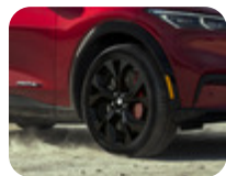
Alloy Wheel 19" 5-spoke Y design, Ebony Black 7 x 19", offset 47.5, for tyres 225/55 R19.
