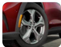
Alloy Wheel 18" 5-spoke Y design, Carbonized Grey 7J x 18", offset 47.5, for tyres 225/60 R18 – up to 08/2023
