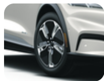
Alloy Wheel 19" 5-spoke Y design, silver 7 x 19", offset 47.5, for tyres 225/55 R19. To be used in combination with Aero Wheel Cover (Finis 2615667). – from 08/2023 onwards
