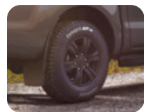
Alloy Wheel 17" 6-spoke design, Asphalt Black 8 x 17", offset 55, for tyres 265/65 R17 – Except Raptor
