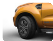
Alloy Wheel 18" 6 x 2-spoke design, Medium Bolder Grey 8 x 18", offset 55, for tyres 265/60 R18 – Except Raptor
