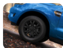
Alloy Wheel 18" 6 x 2-spoke design, Panther Black Single alloy wheel, 8j x 18", offset 55, 265/60 R18 tyre (not included)
