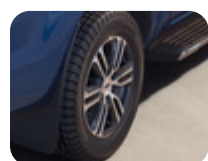
Alloy Wheel 18" 6 x 2-spoke design, Medium Bolder Grey Machined 8 x 18", offset 55, for tyres 265/60 R18 – Except Raptor
