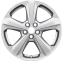
Alloy Wheel 18" 5-spoke design, sparkle silver Single alloy wheel, 7.5j x 18", offset 55, fit with 235/60 R18 tyre
