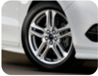
Alloy Wheel 18" 5 x 2-spoke design, sparkle silver Single alloy wheel, 7.5j x 18", offset 55, fit with 235/60 R18 tyre
