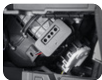
Air Purifier The Ford Air Purifier helps improve the air quality within the cabin by removing small harmful airborne particles. It generates and releases millions of negatively charged particles called ions, these attract and attach themselves to positively charged ions carrying allergens which then become too heavy and fall to the floor. This is designed to neutralize and help remove pollen, pet dander, odours, cigarette smoke and dust, leaving the cabin feeling fresh.
