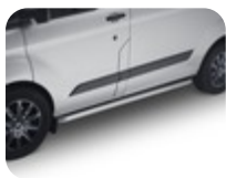
ARP* Side Protection Bar polished stainless steel tubular design with corner bends Set of 2 tubular side protection bars. Electro-deposit primer (EDP) coating black for corrosion prevention. Installation requires no drilling. Length: 2450 mm, diameter: 60 mm by 1.5 mm of wall thickness. Made from ST304 stainless steel and mounting brackets made from ST052 steel. – Vehicles with short wheel base. Except Sport Van
