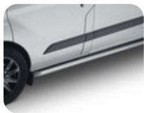
ARP* Side Protection Bar polished stainless steel tubular design Set of 2 tubular side protection bars. Electro-deposit primer (EDP) coating black for corrosion prevention. Installation requires no drilling. Length: 2450 mm, diameter: 60 mm by 1.5 mm of wall thickness. Made from ST304 stainless steel and mounting brackets made from ST052 steel. – Vehicles with long wheel base. Except Sport Van
