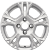
Alloy Wheel 15" 5-spoke design, sparkle silver Single alloy wheel, 6j x 15", offset 47.5, fit with 195/55 R15 tyre – Except ST
