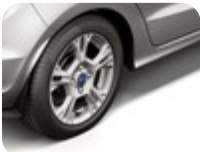
Alloy Wheel 14" 5 x 2-spoke design, sparkle silver Single alloy wheel, 5.5j x 14", offset 37.5, 175/65 R14 tyre (not included)
