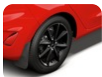
Alloy Wheel 16" 8-spoke design, Black Single alloy wheel, 6.5j x 16", offset 47.5, fit with 195/55 R16 tyre
