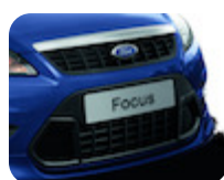
Front Grille lower grille insert in dark grey Lower part radiator grille with unique mesh pattern
