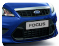
Front Grille upper part With unique mesh pattern, pattern matches lower grille insert
