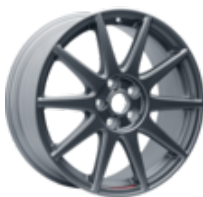
Performance Wheel 18" lightweight Ford Performance alloy wheel Single 18" lightweight flow-form 10 spoke alloy wheel, 8j x 18", 10 spoke design, magnetite matt finish, offset 55 excludes; Tyre, Valve, Centre Cap and Wheel Nuts. Only in combination with steering rack limiter – Only for vehicles equipped with factory fitted 18" wheels (steering rack limiter fitted as standard). Excludes Active
