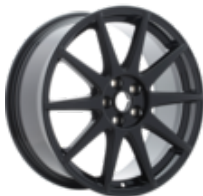
Performance Wheel 19" lightweight flow-form, 10-spoke design, Absolute Black 8 x 19", offset 55, for tyres 235/35 R19. Only in combination with steering rack limiter – ST
