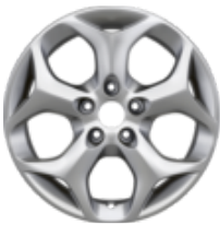
Alloy Wheel 16" 5-spoke Y design, silver Single alloy wheel, 7j x 16", offset 50, fit with 205/55 R16 tyre
