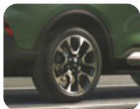
Alloy Wheel 19" 5 x 2-spoke design, Machined Absolute Black 7.5 x 19", offset 50, for tyre 225/55 R19 – Active and Active X
