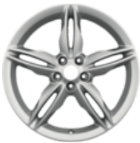
Alloy Wheel 19" 5 x 2-spoke design, silver machined Single alloy wheel, 8j x 19", offset 52.5, fit with 235/45 R19 tyre
