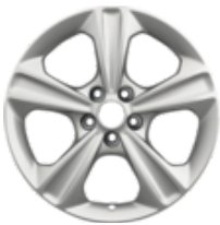
Alloy Wheel 17" 5-spoke design, silver Single alloy wheel, 7.5j x 17", offset 52.5, fit with 235/55 R17 tyre
