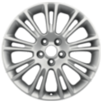
Alloy Wheel 17" 5-spoke design, 'luster nickle' finish Single alloy wheel, 7.5j x 17", offset 52.5, fit with 235/55 R17 tyre
