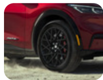
Alloy Wheel 20" 10-spoke X design, Ebony Black 8 x 20", offset 47.5, for tyres 245/45 R20.
