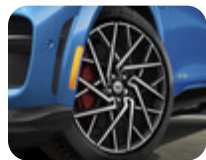
Alloy Wheel 20" 10 x 2-spoke design, Black Machined 8 x 20", offset 47.5, for tyres 245/45 R20 – GT
