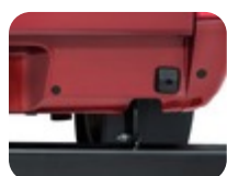
Xvision (SCC)* Parking Distance Sensors rear, with 4 sensors in matt black Provides detection of obstacles, features acoustic warning with increasing intermittent beeping and solid tone at close proximity. Also for vehicles with tow bar or exterior fitted spare wheel. Can be combined with Xvision front parking distance control. Angled sensors with rubber surrounding especially for metal bumpers included in the package allow fitment according to the shape of the bumper. Please note: sensors cannot be painted in body colour. This parking distance control kit comes with an audible signal only and does not integrate with the Ford visual display/SYNC unit. Please ask your Ford Dealer for further details – Except Limited and Wildtrack
