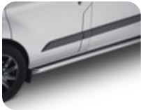
ARP* Side Protection Bar polished stainless steel tubular design
