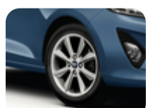
Alloy Wheel 16" 8-spoke design, Sparkle Silver 6.5 x 16", offset 47.5, for tyres 195/55 R16
