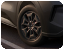
Alloy Wheel 17" 6-spoke design, Magnetic Matt 6.5 x 17", offset 50, for tyres 215/60 R17.
