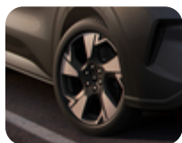
Alloy Wheel 19" 5-spoke design, Asphalt Matt Black 7.5 x 19", offset 52.5, for tyres 235/50 R19.
