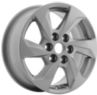
Alloy Wheel 16" 6-spoke design, Sparkle Silver 6.5 x 16", offset 50, for tyres 215/65 R16.
