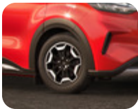
Alloy Wheel 17" 6-spoke design, Ebony Black 6.5 x 17", offset 50, for tyres 215/60 R17.
