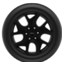
Light Alloy Complete Winter Wheel 17" 5-spoke design, Asphalt Matt Black 6.5J x17 ET50, Nokian Snowproof C, 215/60 R17C 109/107T, label for tyre characteristics according to EU directive no. 2020/740. – With tyre pressure monitoring sensors.
