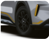
Alloy Wheel 16" 6-spoke design, Asphalt Matt Black 6.5 x 16", offset 50, for tyres 215/65 R16.
