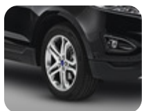
Alufelg 19" 5 x 2-eikers design, Sparkle Nickel 8 x 19", innpress 52,5, for dekk 235/55 R19
