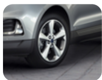
Alufelg 19" 5-eikers design, Sparkle Silver 8 x 19", innpress 52,5, for dekk 235/55 R19
