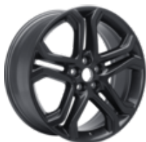
Alufelg 19" 5 x 2-eikers design, premium lakkert aluminium 8 x 19", innpress 52,5, for dekk 235/55 R19
