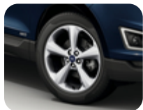
Alufelg 18" 5-eikers design, Sparkle Silver 7,5 x 18", innpress 55, for dekk 235/60 R18
