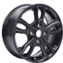
Alufelg 15" 5 x 2-eikers design, Panther Black 6J x 15", innpress 47,5, for dekk 195/55 R15 – Untatt ST
