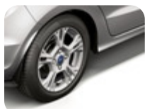
Alufelg 14" 5 x 2-eikers design, Sparkle Silver 5,5 x 14", innpress 37,5, for dekk 175/65 R14 – Untatt ST
