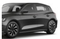
Alufelg 17" 10-eikers design, Absolute Black Machined 7 x 17", innpress 50, for dekk 215/50 R17 91V – Unntatt Active
