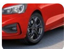
Alufelg 17" 5 x 2-eikers Y-design, Silver Premium 7 x 17", innpress 50, for dekk 215/50 R17 91V – Unntatt Active
