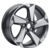
Alufelg 17" 5-eikers design, Silver Premium 7 x 17", innpress 45, for dekk 215/55 R17 94H – Active
