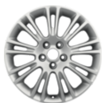
Alufelg 17" 9 x 2-eikers design, Luster Nickel 7,5 x 17", innpress 52,5, for dekk 235/55 R17
