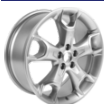
Alufelg 19" 5-eikers Star-design, Luster Nickel 8 x 19", innpress 52,5, for dekk 235/45 R19
